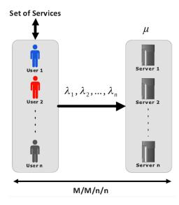
Figure 1. Erlang-Loss System (ELS).
