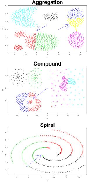
Fig. 11. Three experimental results applying **K-means**, using the classical algorithm <sup>51</sup>. From top to bottom: "Aggregation", "Compound" and "Spiral". The arrows point the problematic sections.
