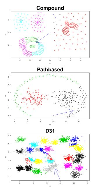
Fig. 10. Three experimental results applying **SC**, using the approach given by Ng et al. <sup>57</sup>. From top to bottom: "Compound", "Pathbased" and "D31". The arrows point the problematic sections.
