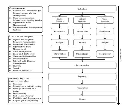
Figure 9: Overall view of DFIPM
