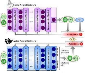
Fig. 3: CACLA-based RL controller architecture.
