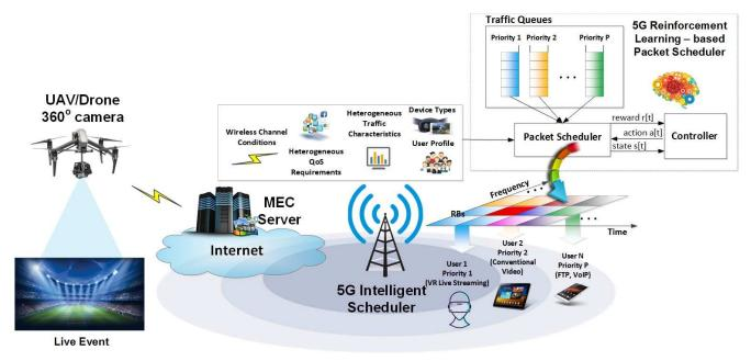
Fig. 2: Proposed 5G UAV-based live streaming framework.
