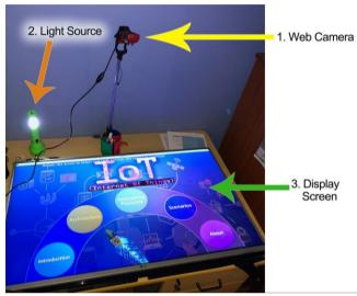
Figure 8 - Physical Setup of System
