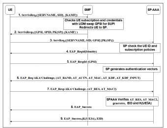
Figure 5 SAP-AKA Protocol Message Exchange Flow
