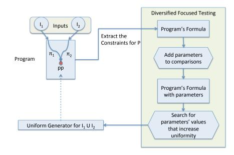
Fig. 1. DFT extracts the program constraints to reach program point *pp*. These are represented as a *program's formula*. It afterwards parametrises the formula. Once parameters are included into the formula, it creates a generator for finding suitable values for these parameters, with a twofold goal: (1) satisfying the original path constraints; (2) sampling diverse inputs uniformly.
