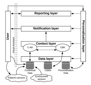
Figure 4.1: The high level architecture of a system built based on ADAPT
