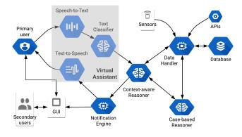
Figure 4.10: Architecture diagram of the system
