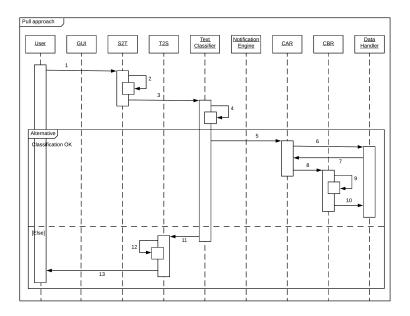
Figure 4.11: Sequence diagram: pull approach
