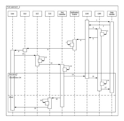
Figure 4.12: Sequence diagram: push approach
