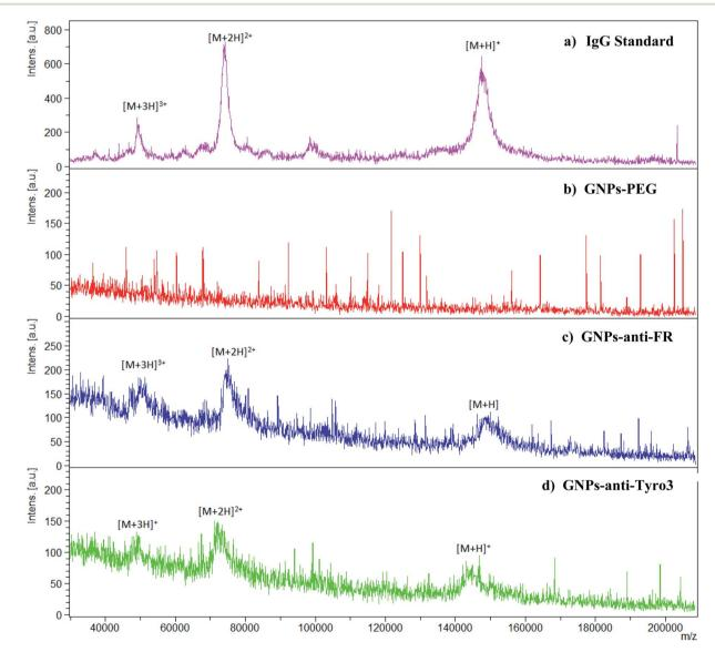
Fig. 6 MALDI-TOF spectra for (a) IgG as the standard, (b) GNPs-PEG, (c) GNPs-anti-FR and (d) GNPs-anti-Tyro3 are shown. High intensity peaks for IgG  $[M + H]^+ = m/z$  148 286,  $[M + 2H]^{2+} = 74$  478 and  $[M + 3H]^{3+}$  are seen. Spectra in (c) and (d) show the same peaks, however, they are absent in GNPs-PEG.
