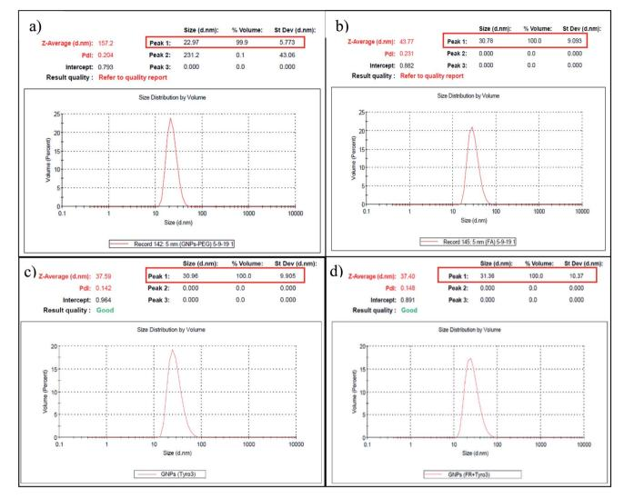
Fig. 4 Hydrodynamic size of GNPs is shown in (a) – (d) of GNPs-PEG, GNPs-anti-FR, GNPs-anti-Tyro3 and GNPs-anti-(FR + Tyro3), respectively. PDI <0.03. The corresponding molecular weights are shown in Fig. 6 and 7.
