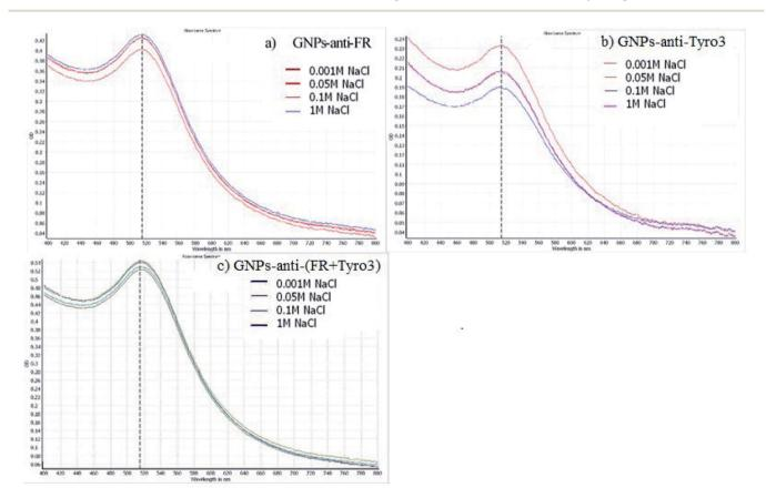
Fig. 3 The stability of (a) GNPs-anti-FR (b) GNPs-anti-Tyro3 and (c) GNPs-anti-(FR + Tyro3) at different NaCl concentration solutions (0.001 M -1 M). UV-vis peak shows no red-shift or broadening of the peak. For each UV-vis spectrum, X-axis represents the wavelength in nanometres (nm) and Y-axis represents the Optical Density (OD).
