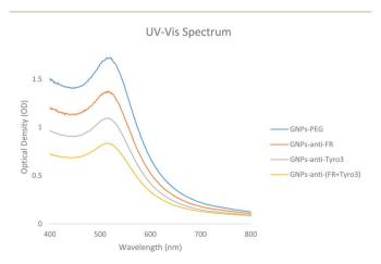
Fig. 2 UV-vis spectra of all 4 GNP constructs GNPs-PEG, GNPs-anti-FR, GNPs-anti-Tyro3 and GNPs-anti-(FR + Tyro3).
