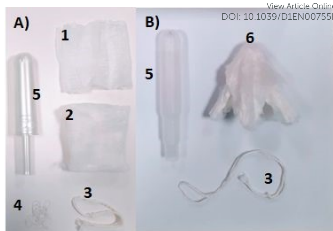
Figure 2 Main types of products found A) comprising a separate cover, B) products not comprising a cover. 1=cover, 2=core, 3=outer string, 4=inner string, 5=applicator and 6=core with no cover
