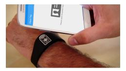
Fig. 2. Silicone Bracelet with NFC Scan screen
