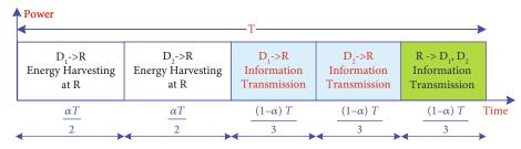
FIGURE 3: The TSR-based R protocol of EH and IP.
