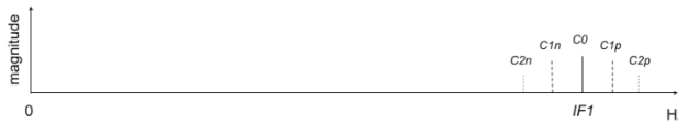
FIGURE 7. RX signal after generic TMA operation – beam harmonics for phased array use created.
