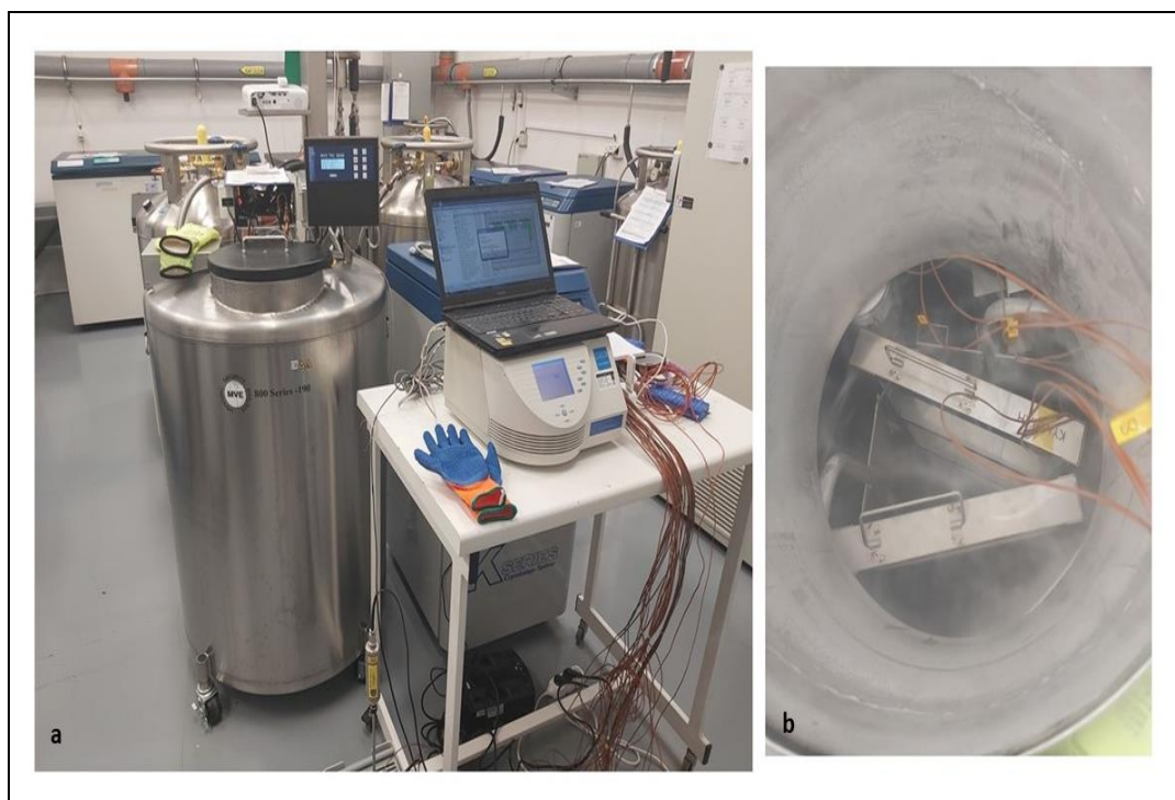
Figure 6. Installation, operational and process qualification performed by the supplier company.
