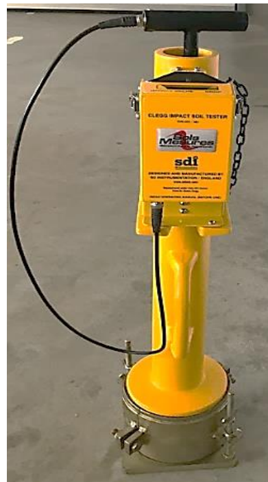
Figure 6. Clegg Impact Soil Tester on cob samples at different water contents.
