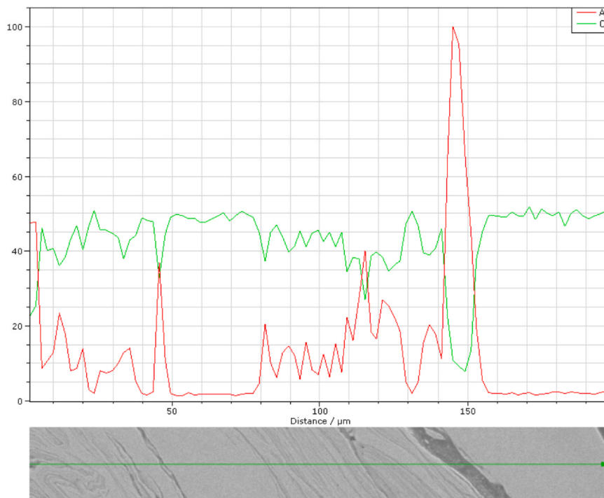
Fig. 14. Line EDX result from the area shown by rectangle in Fig. 13.
