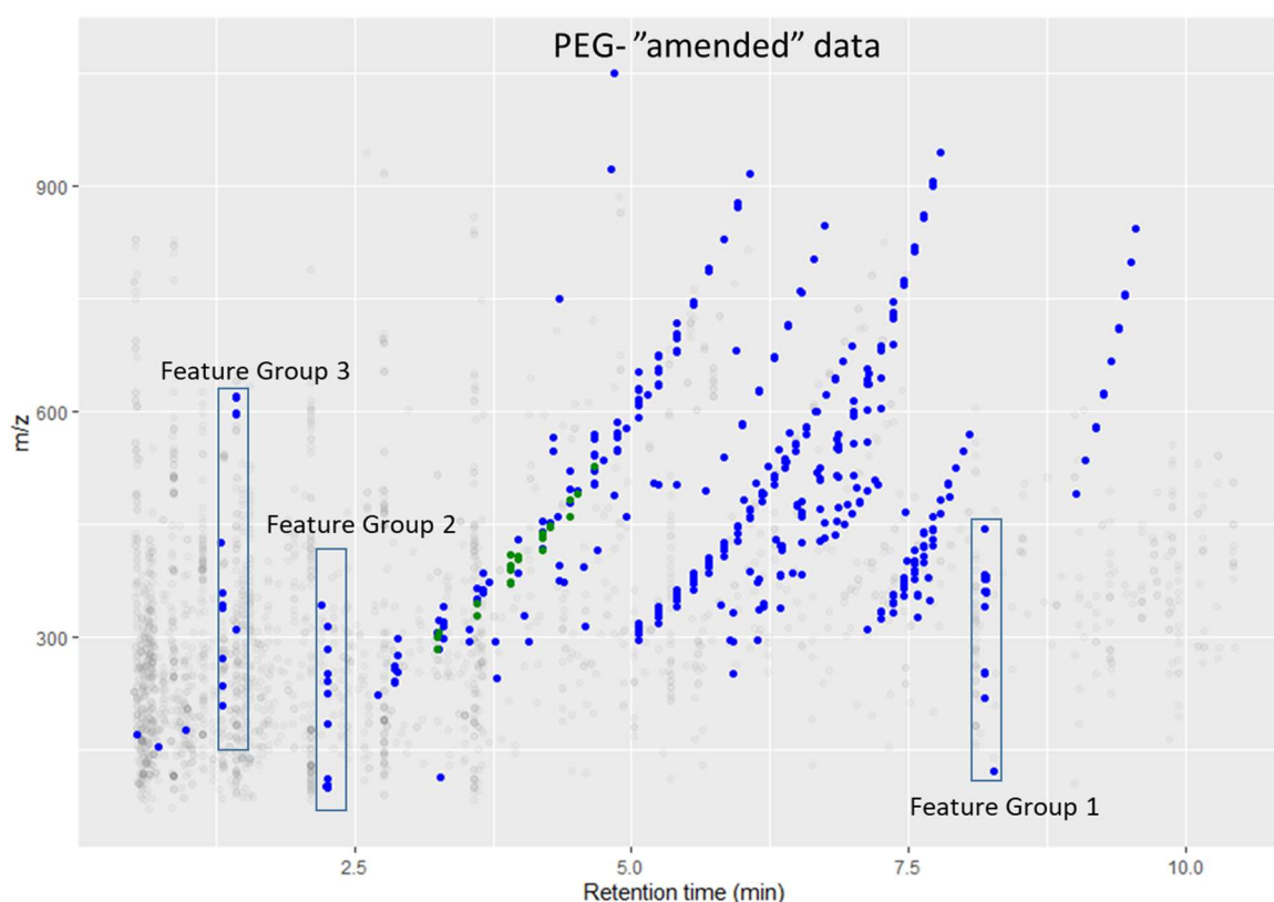
Figure 5-22. Intersample correlation using PEG(n8)-unmetabolised as the driver, observed in the ALZ serum analysed by RPC-UPLC-MS (positive ion mode). Results from the intersample correlation were presented as a retention time (RT) vs m/z plot, where features that correlated to the driver feature (PEG(n8)-unmetabolised), were coloured by statistical significance ( p_{\text{adj}} \leq 0.05 )- blue, and a statistically significant correlation coefficient
