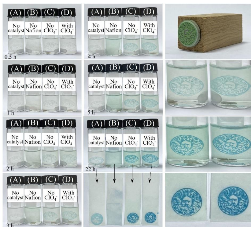
Figure 6.17 Effects of Nafion ionomer printed on a filter paper on the TMB colour response with/without 50 mM \text{ClO}_4^- for 10 mM \text{HCOOH}/\text{HCOONa} concentration at pH 3.75. Photographs of 580 \mu\text{M} TMB (A) without catalyst, (B) without Nafion, (C) in the absence of \text{ClO}_4^- , and (D) with \text{ClO}_4^- (stirred in the dark, 33% DMSO, 11 \text{cm}^3 ) as a function of reaction time.
