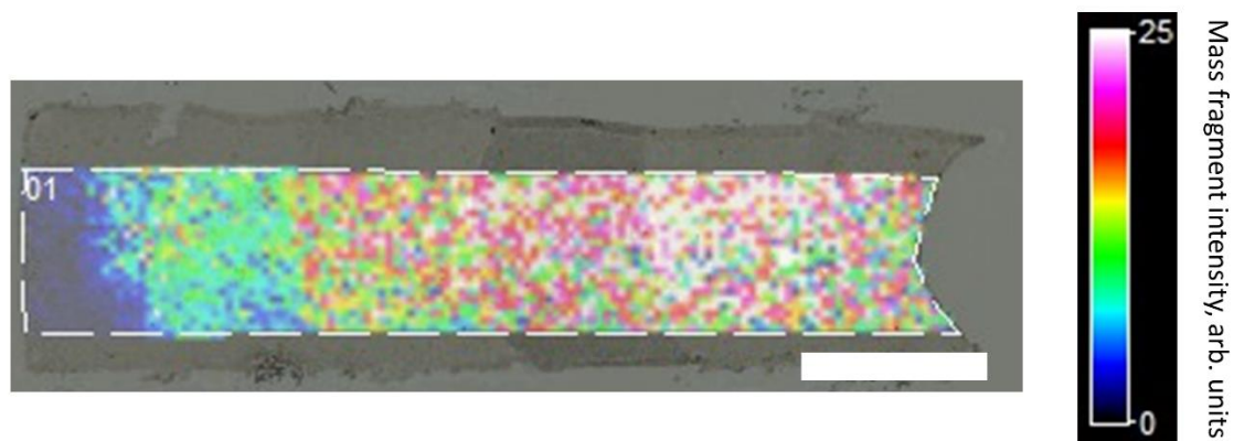
Figure 19: Mimetic tissue model of GSK4 in rat liver, at concentrations of 0, 100, 200, 300, 400, and 500 \mu g/g. MALDI map of mimetic tissue model, with associated colour scale bar, overlaid onto brightfield scan of mimetic tissue. 250.6 Da mass fragment corresponding to the pyrrolidine, phenyl, and alkyne group, used to generate image. Scale bar represents 5 mm.
