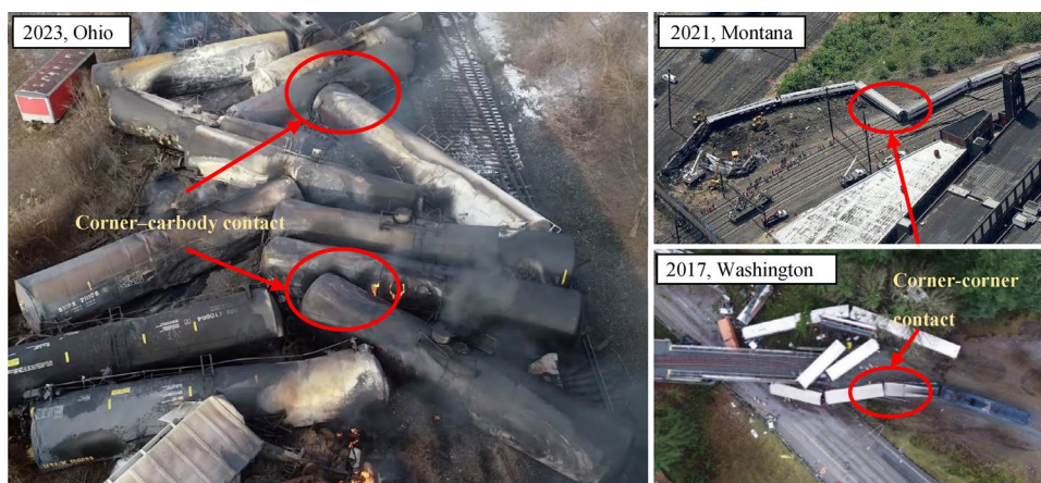
Fig. 4 Two typical contact–impact behaviours between the car bodies
