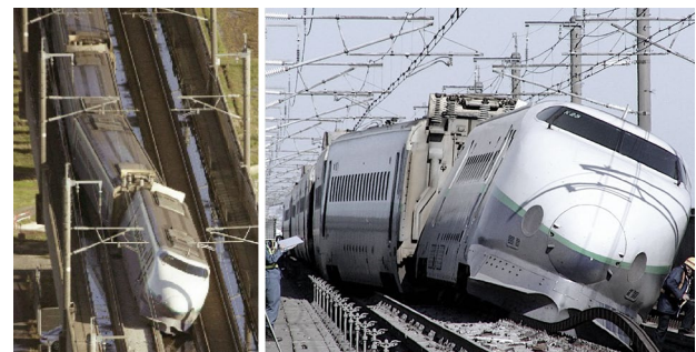
Fig. 2 The derailment accident of a Shinkansen train, in operation since 1964, which highlighted the need for increased focus on train post-derailment studies in both academic and industrial sectors [7]
