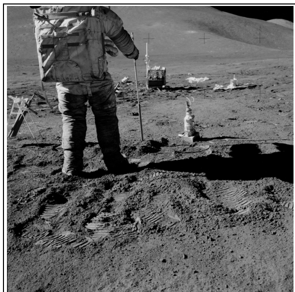
Figure 2: Manual deployment of an Apollo 15 heat flow probe into a predrilled borehole. The drill is shown next to the bore stem.
