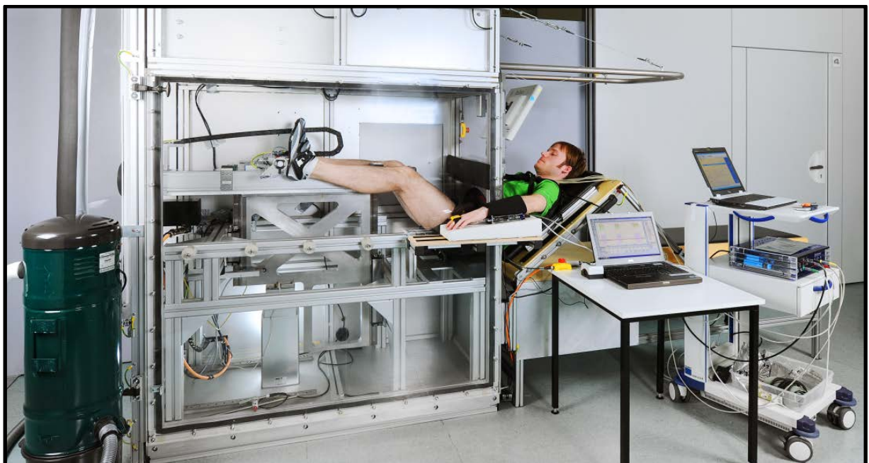
Fig. 15: Position of the subject into the LBNP chamber of the robotic controlled leg press. A vacuum cleaner (left side) realises a pressure difference up to -60 mmHg within the chamber (picture by Evi Blink and Mareike Knost, DLR).
