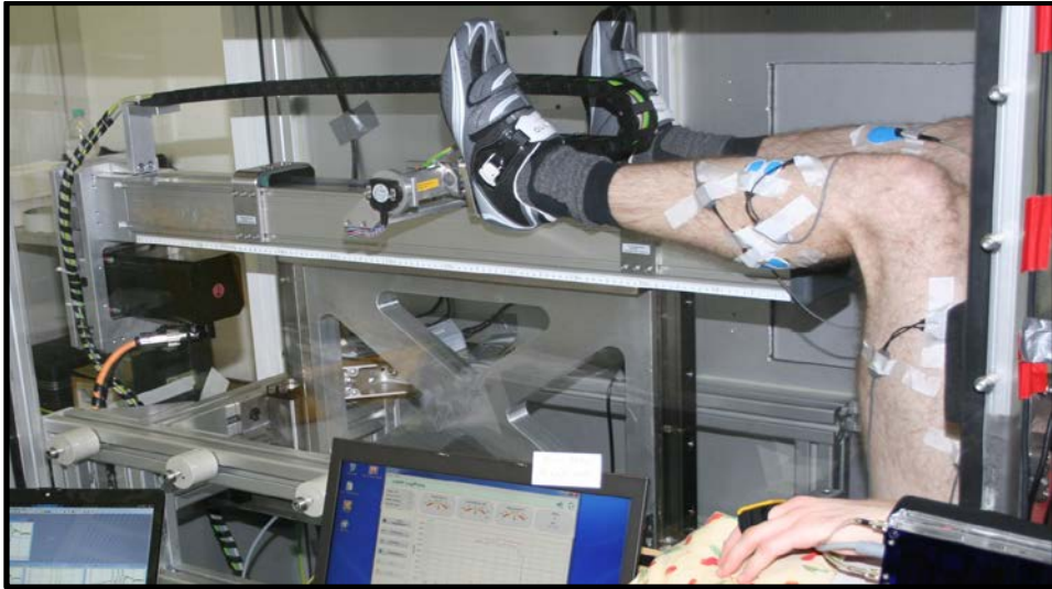
Fig. 13: Proper position of the legs, which are connected via bicycle click shoes to the axis of the linear actuator.
