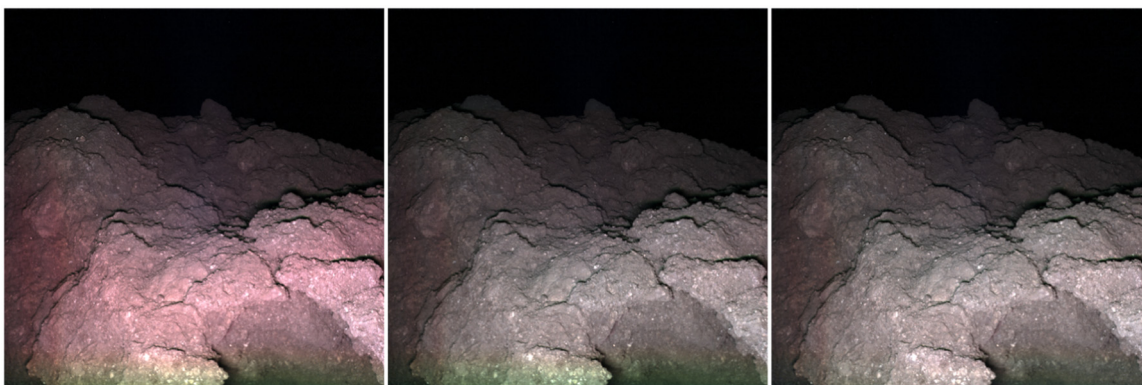
Figure 4. Color correction of the (red, green, blue) = ( R , G , B ) composite of set 14 (brightness enhanced). Left: no color correction ( V_i = 1 ). Middle: colors corrected using the V_i in Figure 19 in Jaumann et al. (2017). Right: colors corrected using the V_i in Figure 3.
