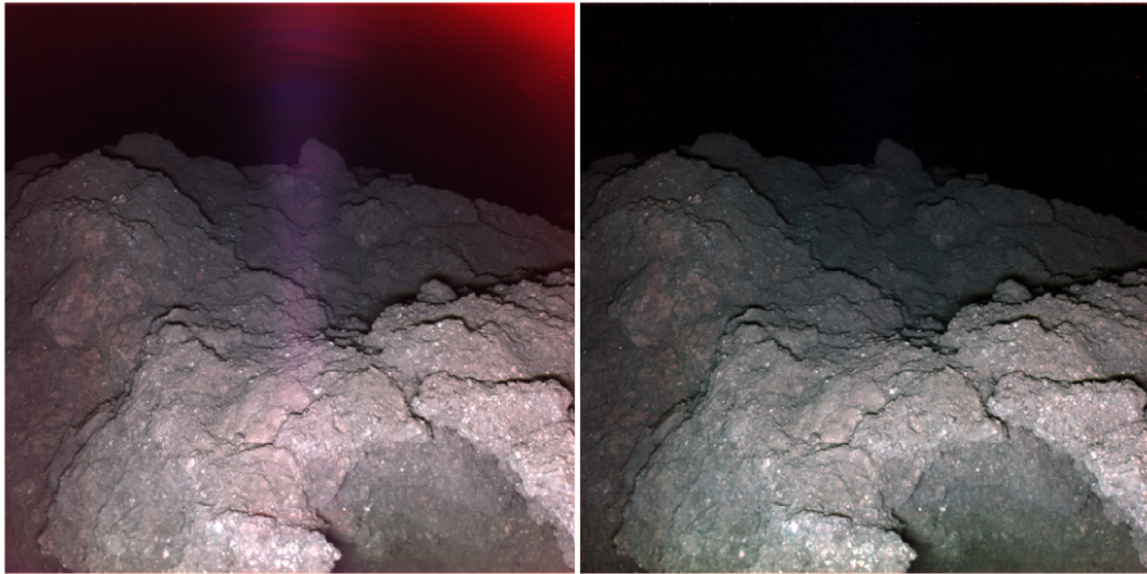
Figure 2. LED stray light correction for the (red, green, blue) = (I, G, B) composite of set 14. Left: without correction. Right: with correction. The brightness of both composites is enhanced identically.
