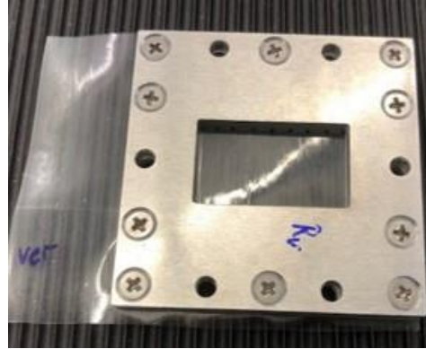
Fig. 4 Plate holder with rectangular cut out and flexible wall
