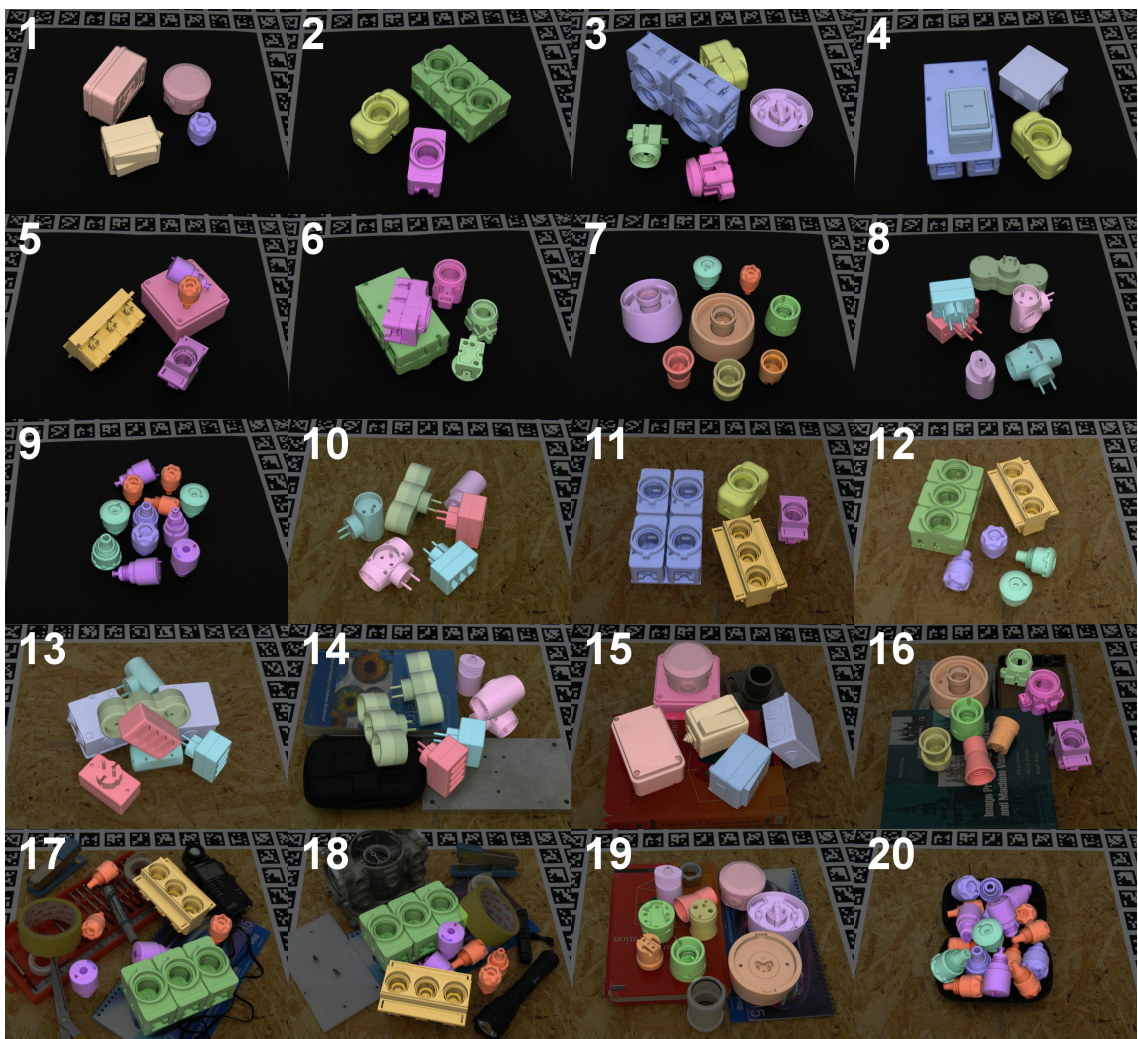
Figure 5.8: Test scenes overlaid with colored 3D object models at ground truth poses
