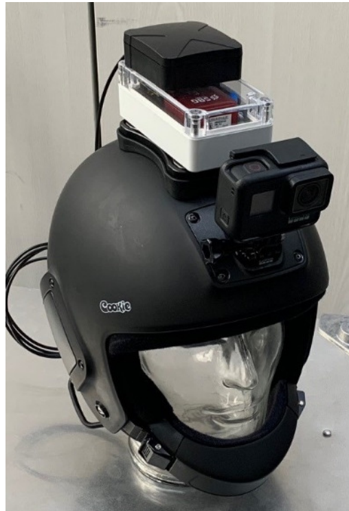
Figure 5. Helmet equipped with a multi-frequency GNSS antenna, integrated navigation system and data recording unit
