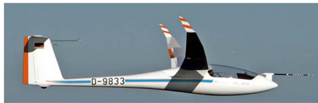
Fig. 13 DLR Discus-2c Sailplane as flight-test platform for loads data generation.
