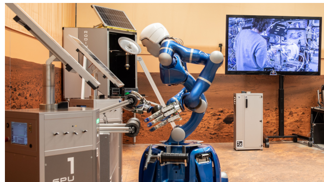
Figure 1. During the first Surface Avatar preliminary experiment session in June 2022, DLR's humanoid robot Rollin' Justin was teleoperated from the International Space Station (ISS). The display in the back shows ESA astronaut Samantha Cristoforetti testing force-reflection teleoperation.
