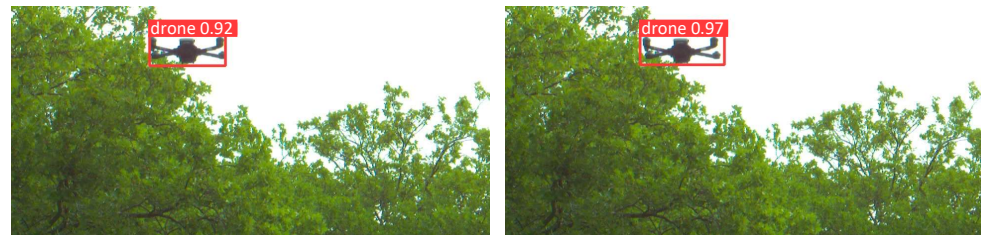
Figure 1. Assessment of the detection accuracy. A comparison of the detection results on real data obtained with model M_S trained solely on synthetic data ( left ) and model M_R trained on real data only ( right ). Both models exhibit a comparable level of confidence in detecting the drone.
