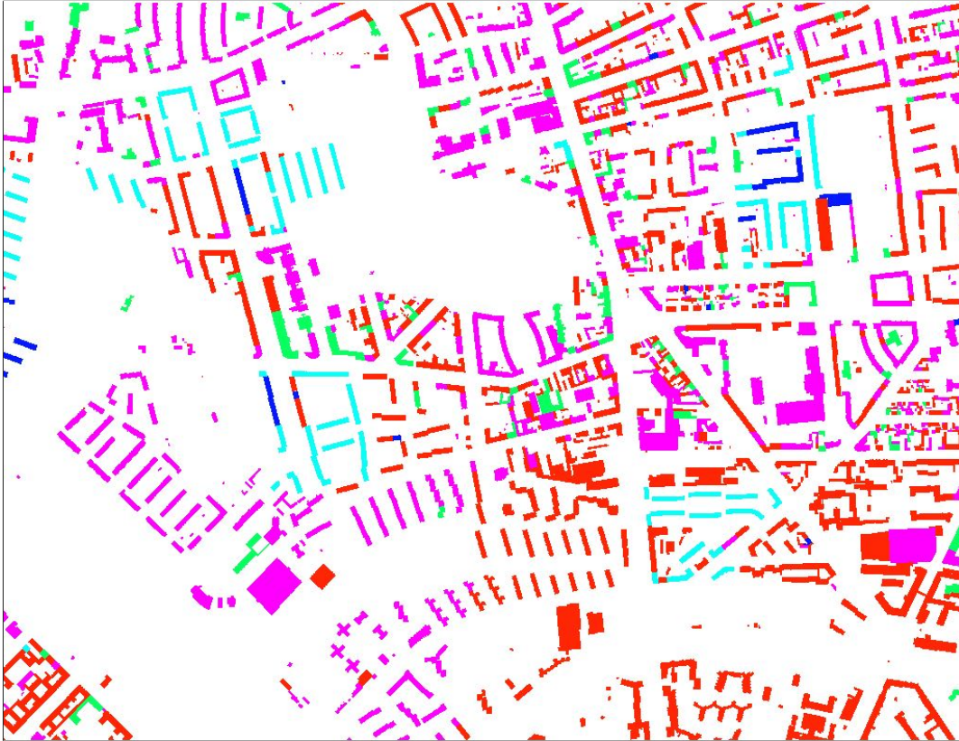
Figure 7: A small area of the ground truth with additionally labeled gable and hip roofs. White: background, magenta: mono-plane, blue: gable, cyan: hip, green: other, red: unknown.
