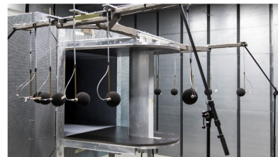
Figure 8: Experimental setup for the BTEN study with DU93W210 airfoil section. The microphones are placed at a distance of 3.3c_b ( c_b refers to the chord length of the unmodified airfoil with t^* = 0.005 ) and rotate with the AoA, thereby keeping their relative positions.
