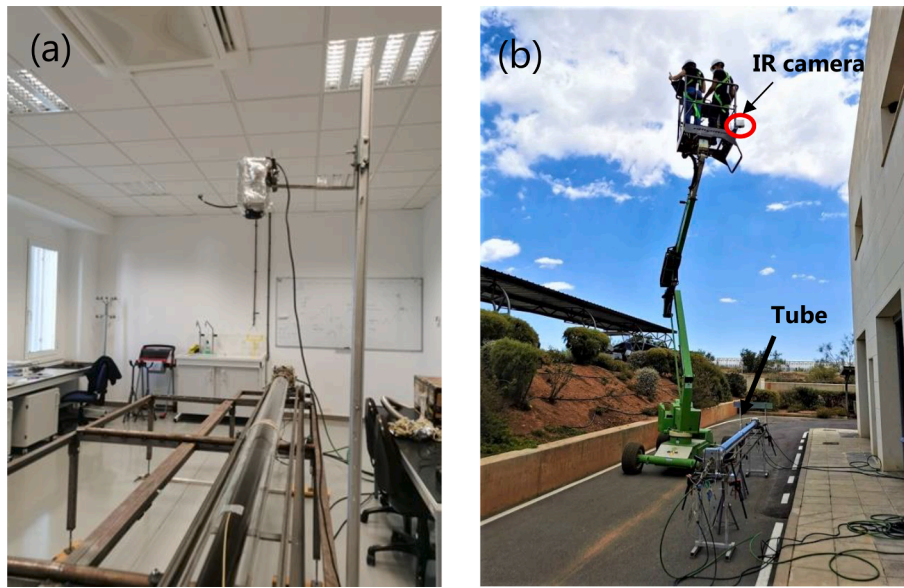
Fig. 2. Experimental device to determine the influence of the camera-source distance on temperature measurement with infrared cameras. Left. Tests in the tube characterisation laboratory of the Plataforma Solar de Almería. Right. Outdoor tests at higher altitudes.
