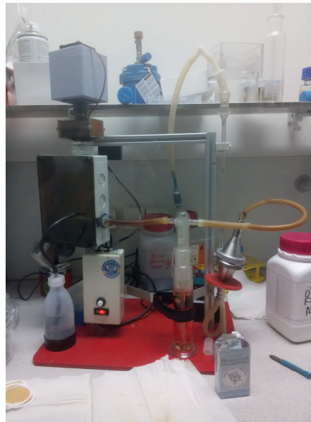
Figure M1: Pump for the generation of cigarette smoke extract
