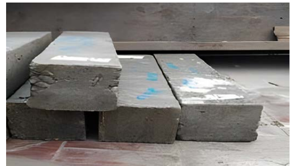
Figure 6: Reinforced concrete beams with PP prepared bars
