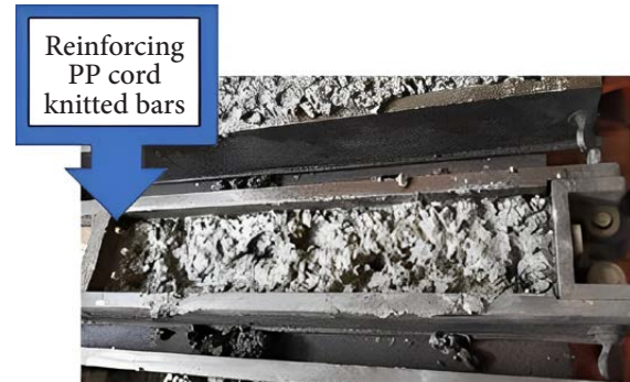
Figure 5: Pouring reinforced beams with PP prepared bars
