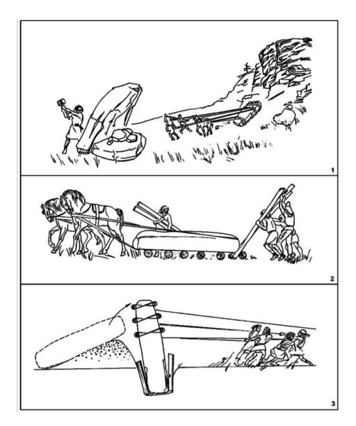
**Figure 2.** Salbyk: 1 – reconstruction of extraction and initial processing of stone slabs in Kyzyl-Khaya; 2 – one of ways of transportation of the slab; 3 – reconstruction of process of installation of vertical the stone slab.
