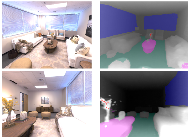
Fig. 1: Our approach grounds open-vocabulary language-based queries in 3D space: • “vacuum the rug”, • “clean the table”, • “pick up the plant”, • “dust the blinds”. The colors indicate the areas in the encoded 3D space that correspond to each command.
