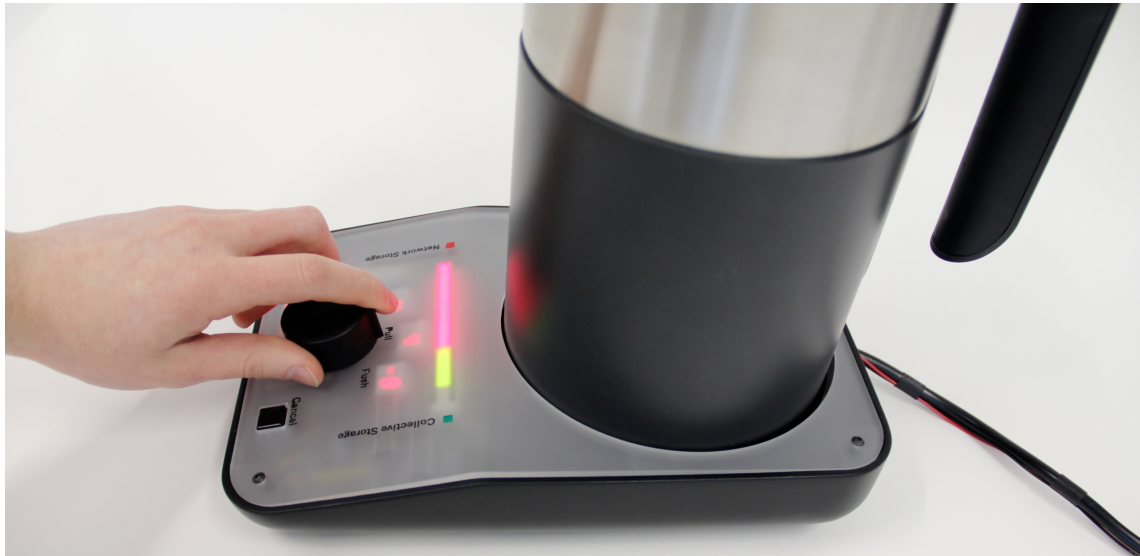
Fig. 1. Karma Kettle: accumulate variable "karma points" by choosing to store, share or use energy according to different contexts
