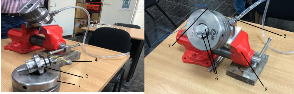
Fig. 2. System configuration: 1 – closed vessel body; 2 – locker; 3 – closed vessel cap; 4 – propellant charge; 5 – exhaust valve; 6 – electrical terminals for firing; 7 – pressure transducer; and 8 – fastening system.
