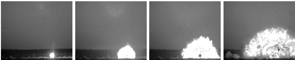
Fig. 12. The sequence of images presenting the expansion of a sphere of heated detonation products; the last frame shows the sphere with a radius of approx. 7 m
