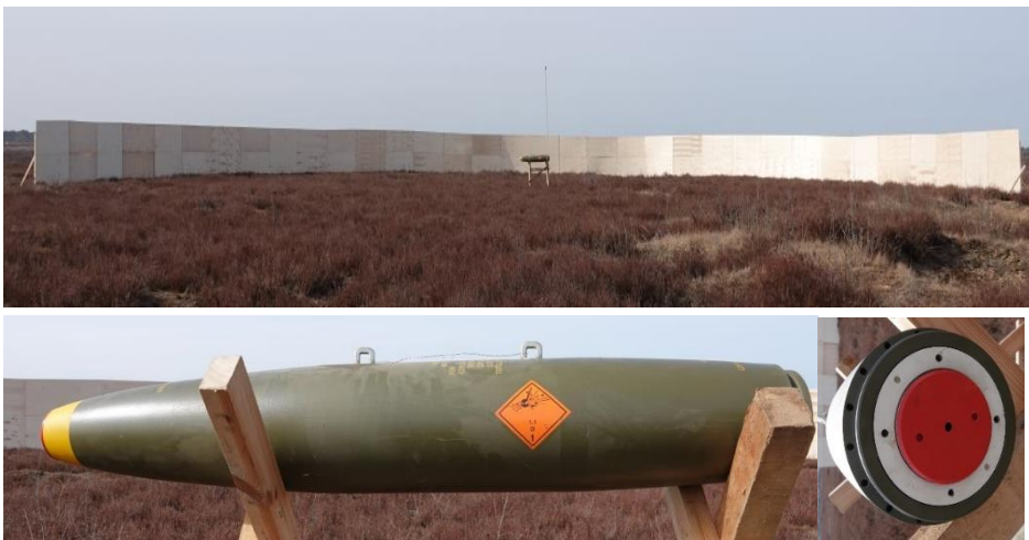
Fig. 1. Range test stand to study the fragment flight geometry and the fragment weight and geometric parameters — general view
