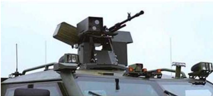
Fig. 2. Remotely controlled, integrated weapon platform. (Photo: author's archive.)
