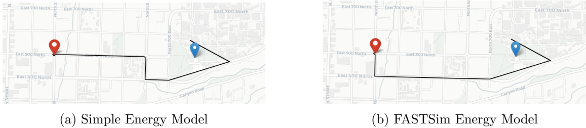
Fig. 5.2: Comparison between Simple and FASTSim Energy Model. FASTSim considers factors throughout the drive cycle and street-dependent acceleration profiles. The simplified physics model assumes vehicle constant acceleration profiles.
