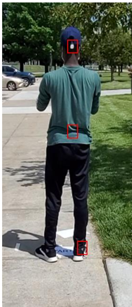
Figure 2. Placement of sensors at three locations on a subject.
