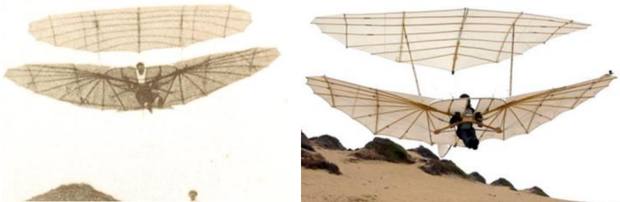
Figs. 13 and 14: Otto Lilienthal piloting one of his gliders (left) and a member of a research team piloting a recreation of the same glider design (right). The aim of the research team was to analyze the process of recreating and piloting one of Lilienthal's gliders, and they were able to achieve several successful flights with minor adjustments made to maximize safety. 53
