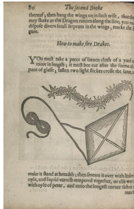
Fig. 2: A depiction of a kite from the seventeenth century English text Mysteries of Nature and Art , which details instructions for making a kite under the title: “How to Make Fire Drakes.” 15 This is one of the first depictions of a kite in print.
