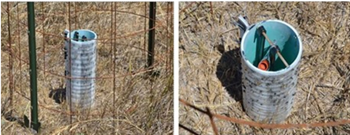
Figure 3. Views of a stable fly trap consisting of a white plastic pipe surrounded with a clear sticky wrap and with an olfactory lure suspended on the inside. Protective fencing surrounding the trap to minimize cattle damage also is shown.
