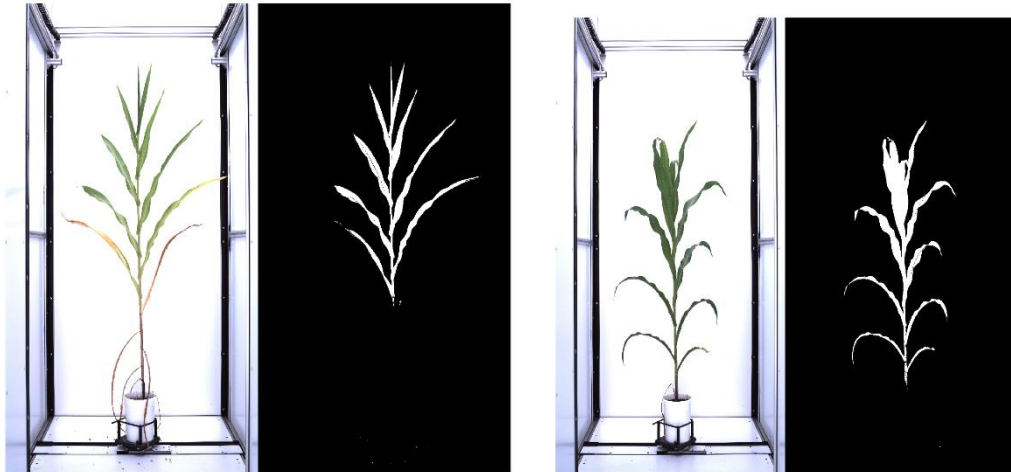
Figure 2.2 Original and binary image after RGB image segmentation in corn
