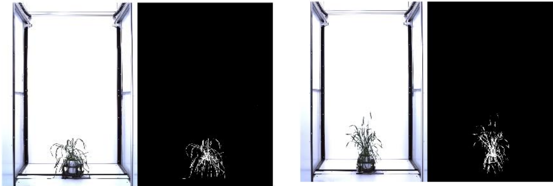
Figure 2.1 Original and binary image after RGB image segmentation in wheat plants
