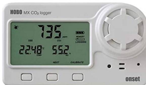
Figure 2 - 3 : Hobo MX1102A CO 2 data logger
