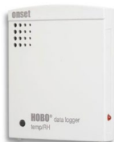
Figure 2 - 2 : HOBO U12 data logger
