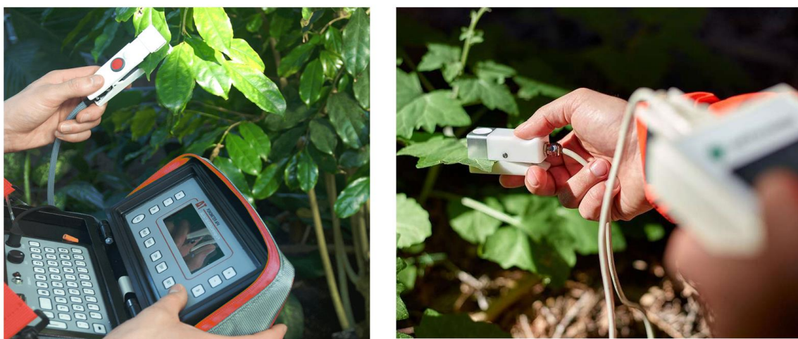
Figure 2: Examples of leaf porometers. Left is AP4 and right is SC-1.
