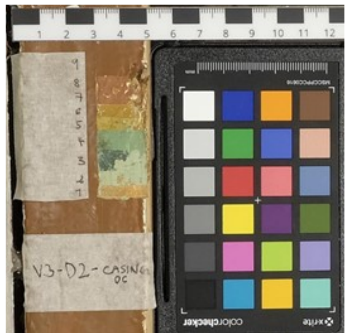
Fig. 3. A paint exposure with the finishes chronologically numbered.
