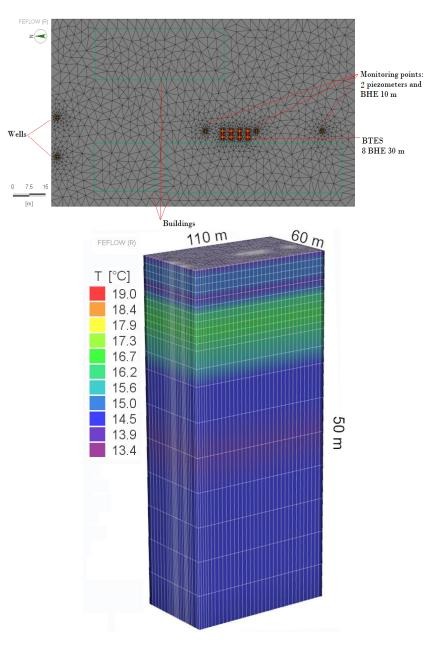
Figure 10. A 3D mesh of the numerical model.
