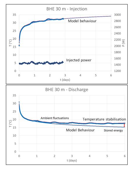
**Figure 5.** Thermal response test conducted over the 30 m deep borehole: injection (**top**) and discharge (**bottom**) phases.
