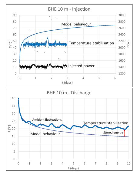
**Figure 4.** Thermal response test conducted over the 10 m deep borehole: injection (**top**) and discharge (**bottom**) phases.
