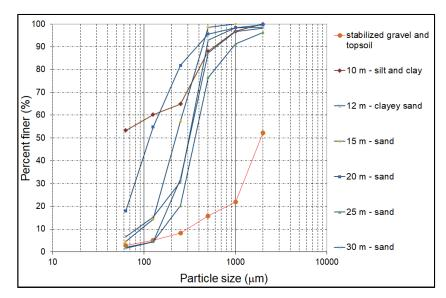
Figure 3. Particle grain size distribution.
