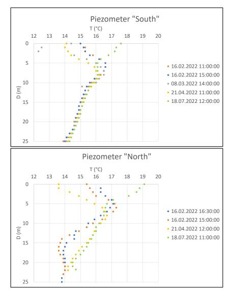
**Figure 6.** Measurements of temperature along depth measured by two piezometers ("South" and "North") in different periods.
