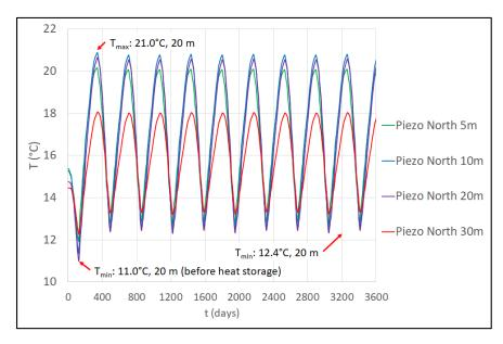
**Figure 15.** The 10-year evolution of the aquifer temperature at the "North" piezometer monitoring point.
