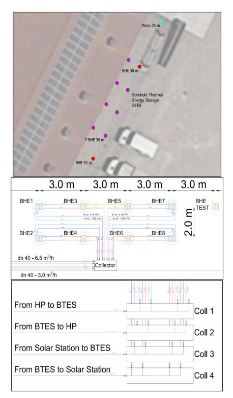
**Figure 9.** Arrangement of the BTES field: aerial photo, scheme of the connections among the BHEs, and scheme of the connections with the collector and details of the four lines.
