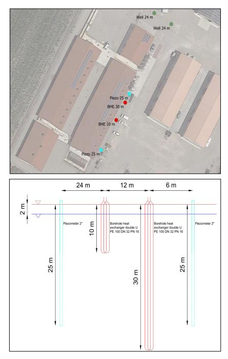
**Figure 8.** Arrangement of borehole heat exchangers and piezometers for preliminary assessment: map and section.
