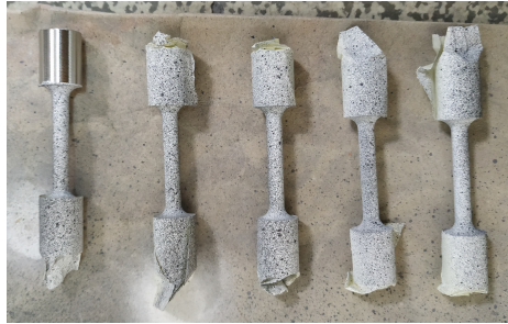
Figure 3.4: Preparation of specimens for tensile test with DIC measurement.
