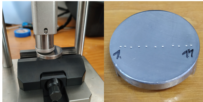
Figure 3.2: UTM test setup (left) and IIT results for the SS304L sample (right).
